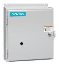
Electrically held lighting contactor, (convertible to mech. held), Amp rating 30A (tungsten 20A), 0 N.C. / 7 N.O. poles, 575-600V 60Hz/550V 50Hz coil, Noncombination type, Enclosure NEMA type 12, Dust/drip proof for indoors
