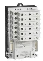
Electrically held lighting contactor, (convertible to mech. held), Amp rating 30A (tungsten 20A), 4 N.C. / 5 N.O. poles, 575-600V 60Hz/550V 50Hz coil, Non-combination type, Enclosure NEMA type (open), No enclosure
