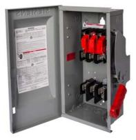
Siemens Low Voltage Circuit Protection Heavy Duty Safety Switches. Type: ENCLOSED, SAFETY SWITCH Std: CSA V. Rating: 600V A. Rating: 100A Wattage: 2W No. Of Poles: 2P F. Rating: 60Hz Action: SINGLE THROW Material: 304SS Enclosure: TYPE 3R. 2-3 point mounting holes. O. Cycles: 10000 O. Temperature: (-20F-120F) AMBIENT TEMPERATURE Environmental Conditions: OUTDOOR
