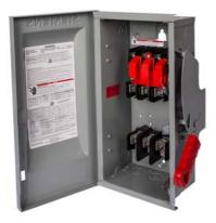
Siemens Low Voltage Circuit Protection Heavy Duty Safety Switches. Type: ENCLOSED, SAFETY SWITCH Std: CUL V. Rating: 600V A. Rating: 100A Wattage: 4W No. Of Poles: 4P F. Rating: 60Hz Action: SINGLE THROW Material: STEEL Enclosure: TYPE 1. 2-3 point mounting holes. O. Cycles: 10000 O. Temperature: (-20F-120F) AMBIENT TEMPERATURE Environmental Conditions: INDOOR
