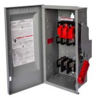
Siemens Low Voltage Circuit Protection Heavy Duty Safety Switch. 3-Pole 3-Wire Fused in a type 3R enclosure (outdoor). Rated 600VAC (200A). Special features: photovoltaic rated, positive ground, 10000 AIC disconnect.
