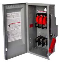
Siemens Low Voltage Circuit Protection Heavy Duty Safety Switches. Type: ENCLOSED, SAFETY SWITCH Std: UL V. Rating: 600V A. Rating: 100A Wattage: 3W No. Of Poles: 3P F. Rating: 60Hz Action: SINGLE THROW Material: STEEL Enclosure: TYPE 1. 2-3 point mounting holes. O. Cycles: 10000 O. Temperature: (-20F-120F) AMBIENT TEMPERATURE Environmental Conditions: INDOOR
