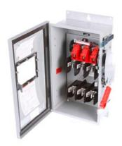
Siemens Low Voltage Circuit Protection Heavy Duty Safety Switches. Type: ENCLOSED, SAFETY SWITCH Std: UL V. Rating: 240V A. Rating: 100A No. Of Poles: 3P F. Rating: 60Hz Action: SINGLE THROW Material: 304SS Enclosure: TYPE 12. 2-3 point mounting holes. Insulation: YES O. Cycles: 10000 O. Temperature: (-20F-120F) AMBIENT TEMPERATURE Environmental Conditions:
