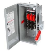
Siemens Low Voltage Circuit Protection Heavy Duty Safety Switches. Type: ENCLOSED, SAFETY SWITCH Std: UL V. Rating: 240V A. Rating: 30 A Wattage: 4W No. Of Poles: 3P F. Rating: 60Hz Action: SINGLE THROW Material: 304SS Enclosure: TYPE 3R. 2-3 point mounting holes. O. Cycles: 10000 O. Temperature: (-20F-120F) AMBIENT TEMPERATURE Environmental Conditions: OUTDOOR
