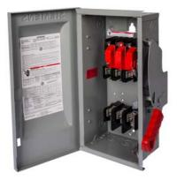
Siemens Low Voltage Circuit Protection Heavy Duty Safety Switches. Type: ENCLOSED, SAFETY SWITCH Std: UL V. Rating: 600V A. Rating: 100A Wattage: 2W No. Of Poles: 2P F. Rating: 60Hz Action: SINGLE THROW Material: 304SS Enclosure: TYPE 3R. 2-3 point mounting holes. O. Cycles: 10000 O. Temperature: (-20F-120F) AMBIENT TEMPERATURE Environmental Conditions: OUTDOOR
