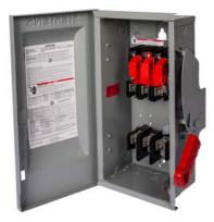
Siemens Low Voltage Circuit Protection Heavy Duty Safety Switches. Type: ENCLOSED, SAFETY SWITCH Std: UL V. Rating: 600V A. Rating: 60A Wattage: 2W No. Of Poles: 2P F. Rating: 60Hz Action: SINGLE THROW Material: STEEL Enclosure: TYPE 1. 2-3 point mounting holes. O. Cycles: 10000 O. Temperature: (-20F-120F) AMBIENT TEMPERATURE Environmental Conditions: INDOOR
