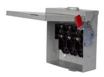
Siemens Low Voltage Circuit Protection Heavy Duty Safety Switches. Type: ENCLOSED, SAFETY SWITCH Std: UL V. Rating: 240V A. Rating: 200A Wattage: 3W No. Of Poles: 2P F. Rating: 60Hz Action: DOUBLE THROW Material: 304SS Enclosure: TYPE 3R. 2-3 point mounting holes. O. Cycles: 8000 O. Temperature: (-20F-120F) AMBIENT TEMPERATURE Environmental Conditions: OUTDOOR
