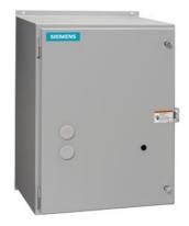
Mechanically held Lighting contactor Contactor amp rating 200Amp 0 NC / 3 NO poles 208VAC 60HZ coil Non-combination type Encl NEMA type 4X 304 S-steel Water/dust tight non-corrosive
