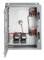
Duplex starter with alternator Size 4 Three phase full voltage Solid-state overload relay OLR amp range 50-200A 110VAC 50Hz / 120VAC 60Hz Coil Combination type Two 200A disconnect switches Enclosure NEMA type 4/12 Water/dust tight weather proof
