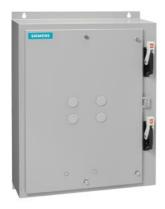
Duplex starter w/o alternator Size 3.5 Three phase full voltage Solid-state overload relay OLR amp range 50-200A 240VAC 50Hz / 277VAC 60Hz Coil Combination type Two 200A disconnect switches Enclosure NEMA type 1 Indoor general purpose use
