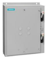
Duplex starter w/o alternator, Size 3 1/2, Three phase full voltage, Solid-state overload relay, OLR amp range 50-200A, 190-220/220-240V 50/60Hz coil, Combination type, Two 125A circuit breakers, Enclosure NEMA type 12, Dust/drip proof for indoors
