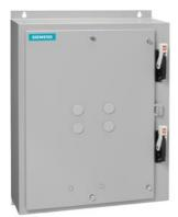
Duplex starter w/o alternator, Size 3 1/2, Three phase full voltage, Solid-state overload relay, OLR amp range 50-200A, 110V 50Hz / 120V 60Hz coil, Combination type, Two 125A circuit breakers, Enclosure NEMA type 12, Dust/drip proof for indoors
