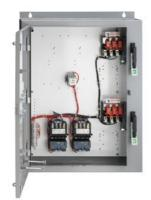
Duplex starter with alternator Size 3.5 Three phase full voltage Solid-state overload relay OLR amp range 50-200A 110VAC 50Hz / 120VAC 60Hz Coil Combination type Two 200A disconnect switches Encl NEMA type 4 painted steel Water/dust tight weather proof
