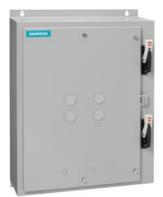
Duplex starter w/o alternator, Size 2 1/2, Three phase full voltage, Solid-state overload relay, OLR amp range 25-100A, 240V 50Hz / 277V 60Hz coil, Combination type, Two 100A circuit breakers, Enclosure NEMA type 12, Dust/drip proof for indoors
