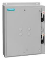
Duplex starter w/o alternator Size 2.5 Three phase full voltage Solid-state overload relay OLR amp range 25-100A 240VAC 50Hz / 277VAC 60Hz Coil Combination type Two 100A disconnect switches Enclosure NEMA type 4/12 Water/dust tight weather proof
