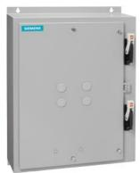
Duplex starter w/o alternator Size 2.5 Three phase full voltage Solid-state overload relay OLR amp range 25-100A 24VAC 50-60Hz Coil Combination type Two 100A disconnect switches Enclosure NEMA type 4/12 Water/dust tight weather proof
