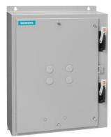
Duplex starter w/o alternator Size 2 Three phase full voltage Solid-state overload relay OLR amp range 13-52A Combination type Two 60A disconnect switches Encl NEMA type 4X 304 S. Steel Water/dust tight non-corrosive
