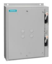
Duplex starter w/o alternator, Size 2, Three phase full voltage, Solid-state overload relay, OLR amp range 13-52A, 110V 50Hz / 120V 60Hz coil, Combination type, Two 50A circuit breakers, Enc NEMA type 4 painted steel, Water/dust tight for outdoors
