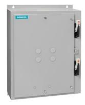
Duplex starter w/o alternator, Size 1, Three phase full voltage, Solid-state overload relay, OLR amp range 5.5-22A, 110V 50Hz / 120V 60Hz coil, Combination type, Two 25A circuit breakers, Enclosure NEMA type 12, Dust/drip proof for indoors
