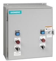
Duplex starter w/ alternator, Size 3 1/2, Three phase full voltage, Solid-state overload relay, OLR amp range 50-200A, 110V 50Hz / 120V 60Hz coil, Non-combination type, Enclosure NEMA type 12, Dust/drip proof for indoors
