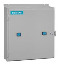
Duplex starter w/o alternator, Size 3, Three phase full voltage, Solid-state overload relay, OLR amp range 25-100A, 380-440/440-480V 50/60Hz coil, Non-combination type, Enclosure NEMA type 12, Dust/drip proof for indoors
