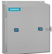
Duplex starter w/o alternator, Size 3, Three phase full voltage, Solid-state overload relay, OLR amp range 25-100A, 190-220/220-240V 50/60Hz coil, Non-combination type, Enclosure NEMA type 12, Dust/drip proof for indoors
