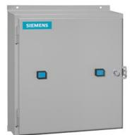
Duplex starter w/o alternator, Size 2 1/2, Three phase full voltage, Solid-state overload relay, OLR amp range 25-100A, 208VAC 60Hz coil, Non-combination type, Enclosure NEMA type 12, Dust/drip proof for indoors
