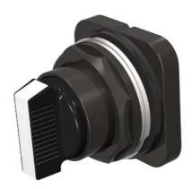
Selector switch, metal, NEMA 4X Spring return left & right Short lever, C Cam 3 position Operator only white insert Non-Illuminated UL file E22655 in Vol. 6 (7) Sec. 13 (2)
