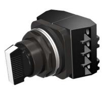
30mm BlackMax, Epoxy Coated Corrosion Resistant Complete Metal Unit Non-Illuminated Selector Switch, Short Lever Black with White Insert 3 Position, C-CAM Spring Return from Left with 2 N.O. - 2 N.C. Heavy Duty Contacts, A600/P600 UL Listed, CSA Certified NEMA 1,3,3R,4,4X,12,13 & Automotive Standards
