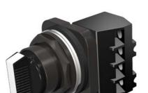
30mm BlackMax, Epoxy Coated Corrosion Resistant Complete Metal Unit Non-Illuminated Selector Switch, Short Lever Black with White Insert 3 Position, C-CAM Spring Return from Left with 1 N.O. - 1 N.C. Heavy Duty Contacts, A600/P600 UL Listed, CSA Certified NEMA 1,3,3R,4,4X,12,13 & Automotive Standards
