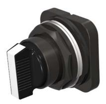
Selector switch, metal, NEMA 4X Spring return left & right Short lever, B Cam 3 position Operator only white insert Non-Illuminated UL file E22655 in Vol. 6 (7) Sec. 13 (2)
