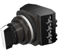
Selector switch, metal, NEMA 4X Maintained Short lever, B Cam 1NC left, 1NO right 3 position Complete device white insert Non-Illuminated UL file E22655 in Vol. 6 (7) Sec. 13 (2)
