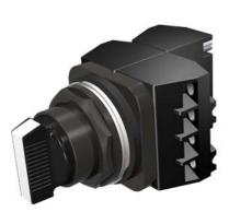
30mm BlackMax, Epoxy Coated Corrosion Resistant Complete Metal Unit Non-Illuminated Selector Switch, Short Lever Black with White Insert 2 Position, A-CAM Maintained with 3 N.O. Heavy Duty Contacts, A600/P600 UL Listed, CSA Certified NEMA 1,3,3R,4,4X,12,13 & Automotive Standards
