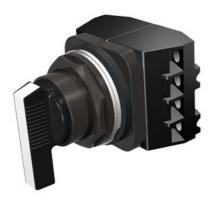
Selector switch, metal, NEMA 4X Spring return left & right Long lever, C Cam 1NO-1NC left, 1NO-1NC right 3 position Complete device white insert Non-Illuminated UL file E22655 in Vol. 6 (7) Sec. 13 (2)
