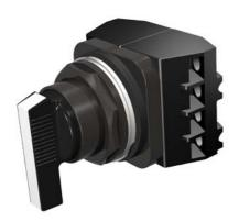
Selector switch, metal, NEMA 4X Spring return from right Long lever, C Cam 1NO-1NC left,1NO-1NC right 3 position Complete device white insert Non-Illuminated UL file E22655 in Vol. 6 (7) Sec. 13 (2)
