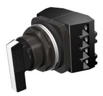
Selector switch, metal, NEMA 4X Maintained Long lever, C Cam 1NO-1NC left, 1NO-1NC right 3 position Complete device white insert Non-Illuminated UL file E22655 in Vol. 6 (7) Sec. 13 (2)
