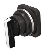
Selector switch, metal, NEMA 4X Maintained Long lever, B Cam 3 position Operator only white insert Non-Illuminated UL file E22655 in Vol. 6 (7) Sec. 13 (2)
