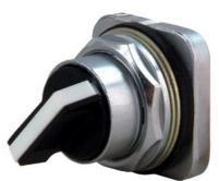
Metal, selector switch Maintained, short lever Position, C Cam 3 position Operator only white insert Non-Illuminated UL file E22655 in Vol. 6 (7) Sec. 13 (2)
