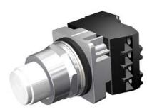
30mm Command/52, Chrome Finish Heavy Duty, Watertight/Oiltight Complete Metal Unit PTT / Illuminated Pushbutton Transformer type, 240V AC Incandescent Lamp Extended Button Plastic Lens, White 2 Position Momentary with 1 N.O. - 1 N.C. Heavy Duty Contacts, A600/P600 UL Listed, CSA Certified NEMA 1,3,3R,4,4X,12,13 & Automotive Standards
