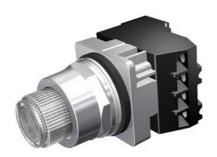
30mm Command/52, Chrome Finish Heavy Duty, Watertight/Oiltight Complete Metal Unit PTT / Illuminated Pushbutton Transformer type, 240V AC Incandescent Lamp Extended Button Plastic Lens, Clear 2 Position Momentary with 1 N.O. - 1 N.C. Heavy Duty Contacts, A600/P600 UL Listed, CSA Certified NEMA 1,3,3R,4,4X,12,13 & Automotive Standards
