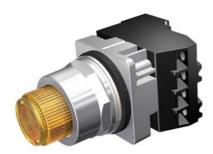
30mm Command/52, Chrome Finish Heavy Duty, Watertight/Oiltight Complete Metal Unit PTT / Illuminated Pushbutton Transformer type, 240V AC Incandescent Lamp Extended Button Plastic Lens, Amber 2 Position Momentary with 1 N.O. - 1 N.C. Heavy Duty Contacts, A600/P600 UL Listed, CSA Certified NEMA 1,3,3R,4,4X,12,13 & Automotive Standards
