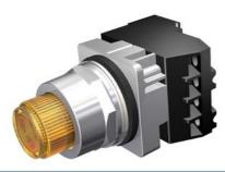
30mm Command/52, Chrome Finish Heavy Duty,Watertight/Oiltight Complete Metal Unit PTT / Illuminated Pushbutton Transformer type, 240V AC LED Lamp Extended Button Plastic Lens, Amber 2 Position Momentary with 1 N.O. - 1 N.C. Heavy Duty Contacts, A600/P600 UL Listed, CSA Certified NEMA 1,3,3R,4,4X,12,13 & Automotive Standards
