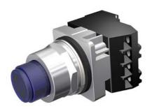
30mm Command/52, Chrome Finish Heavy Duty, Watertight/Oiltight Complete Metal Unit PTT / Illuminated Pushbutton Transformer type, 240V AC LED Lamp Extended Button Plastic Lens, Blue 2 Position Momentary with 1 N.O. - 1 N.C. Heavy Duty Contacts, A600/P600 UL Listed, CSA Certified NEMA 1,3,3R,4,4X,12,13 & Automotive Standards
