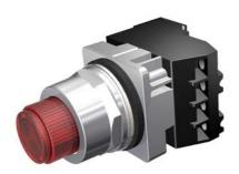
30mm Command/52, Chrome Finish Heavy Duty, Watertight/Oiltight Complete Metal Unit PTT / Illuminated Pushbutton Transformer type, 240V AC LED Lamp Extended Button Plastic Lens, Red 2 Position Momentary with 1 N.O. - 1 N.C. Heavy Duty Contacts, A600/P600 UL Listed, CSA Certified NEMA 1,3,3R,4,4X,12,13 & Automotive Standards
