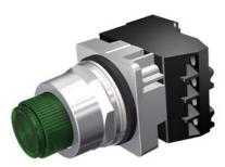
30mm Command/52, Chrome Finish Heavy Duty,Watertight/Oiltight Complete Metal Unit PTT / Illuminated Pushbutton Full Voltage, 6V AC/DC Incandescent Lamp Extended Button Plastic Lens, Green 2 Position Momentary with 1 N.O. - 1 N.C. Heavy Duty Contacts, A600/P600 UL Listed, CSA Certified NEMA 1,3,3R,4,4X,12,13 & Automotive Standards
