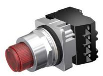
30mm Command/52, Chrome Finish Heavy Duty, Watertight/Oiltight Complete Metal Unit PTT / Illuminated Pushbutton Full Voltage, 6V AC/DC Incandescent Lamp Extended Button Plastic Lens, Red 2 Position Momentary with 1 N.O. - 1 N.C. Heavy Duty Contacts, A600/P600 UL Listed, CSA Certified NEMA 1,3,3R,4,4X,12,13 & Automotive Standards
