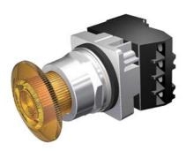
30mm Command/52, Chrome Finish Heavy Duty, Watertight/Oiltight Complete Metal Unit Illuminated Twist-to-Release Full Voltage, 24V AC/DC Incandescent Lamp Mushroom Head Cap Small 1.79" (45 mm) Plastic Cap, Amber 2 Position Maintained, Twist-to-Release with 1 N.O. - 1 N.C. Heavy Duty Contacts, A600/P600 UL Listed, CSA Certified NEMA 1,3,3R,4,4X,12,13 & Automotive Standards
