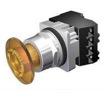
30mm Command/52, Chrome Finish Heavy Duty,Watertight/Oiltight Complete Metal Unit Illuminated Twist-to-Release Full Voltage, 24V AC/DC LED Lamp Mushroom Head Cap Small 1.79" (45 mm) Plastic Cap, Amber 2 Position Maintained, Twist-to-Release with 1 N.O. - 1 N.C. Heavy Duty Contacts, A600/P600 UL Listed, CSA Certified NEMA 1,3,3R,4,4X,12,13 & Automotive Standards
