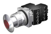
30mm Command/52, Chrome Finish Heavy Duty, Watertight/Oiltight Complete Metal Unit Illuminated Push-Pull Operator Full Voltage, 120V AC/DC Incandescent Lamp Mushroom Head Cap Small 1 3/4" (44.5 mm) Metal, Chrome with Red Lens 3 Position Pull-Momentary/Push-Maintained 1 N.C.+1 N.C. Extra Late Break Heavy Duty Contacts, A600/P600 UL Listed, CSA Certified NEMA 1,3,3R,4,4X,12,13 & Automotive Standards
