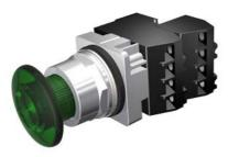
30mm Command/52, Chrome Finish Heavy Duty, Watertight/Oiltight Complete Metal Unit Illuminated Push-Pull Operator Full Voltage, 24V AC/DC LED Lamp Mushroom Head Cap Small 1 3/4" (44.5 mm) Plastic, Green 3 Position Pull-Momentary/Push-Maintained 1 N.C.+1 N.C. Extra Late Break Heavy Duty Contacts, A600/P600 UL Listed, CSA Certified NEMA 1,3,3R,4,4X,12,13 & Automotive Standards
